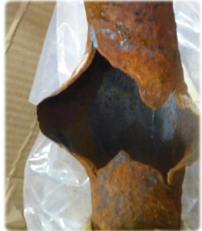
Superheater tube corroded and burst
